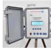
Automatic Stack Monitoring Kits (8 No.s)
