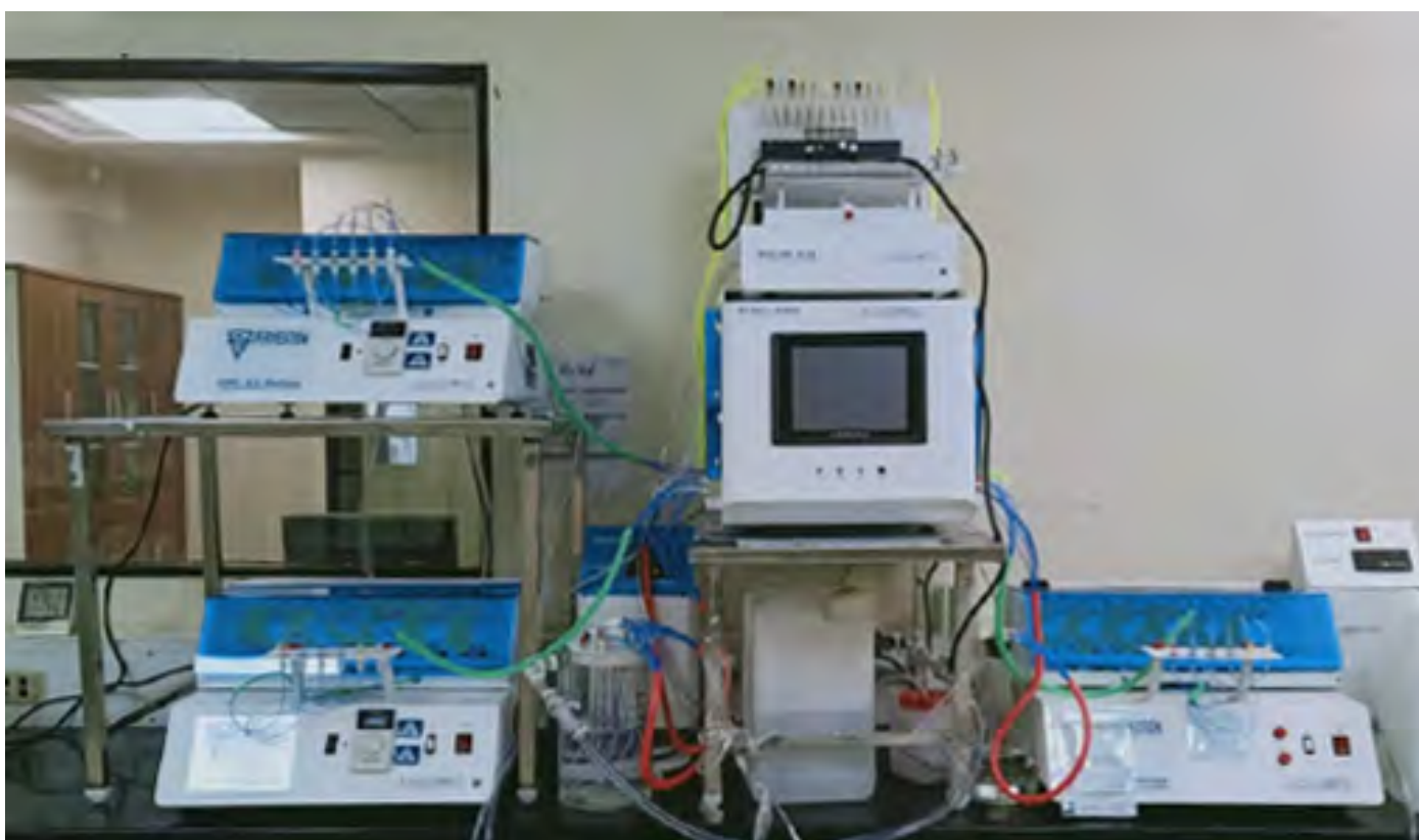
Multi-station Automated Franz Diffusion Cell System at Vimta
